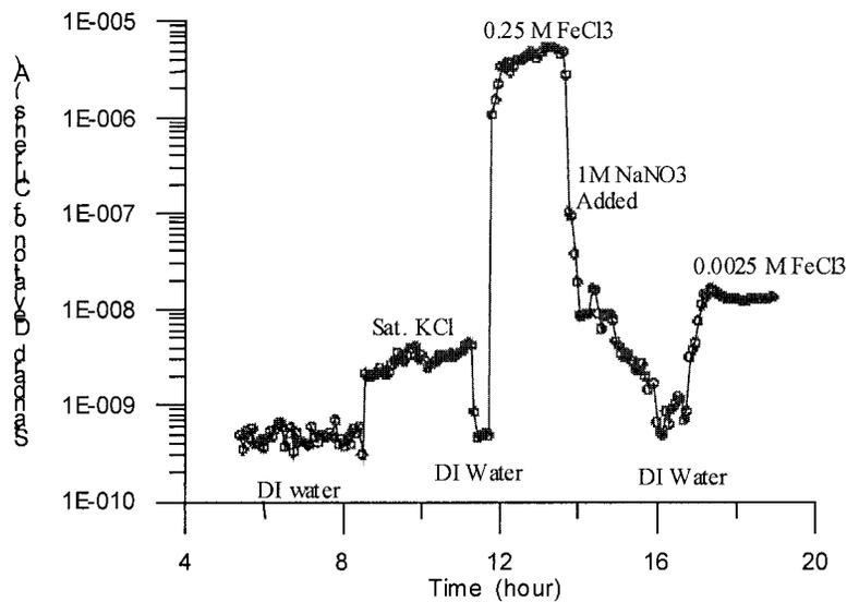
**Figure 3: Typical standard deviation signal of a stainless steel UNS S30400 MASS probe in different localized corrosion environments (from Ref 6)**
