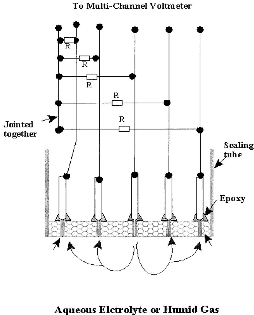
**Figure 1: Schematic of MASS probe.**
