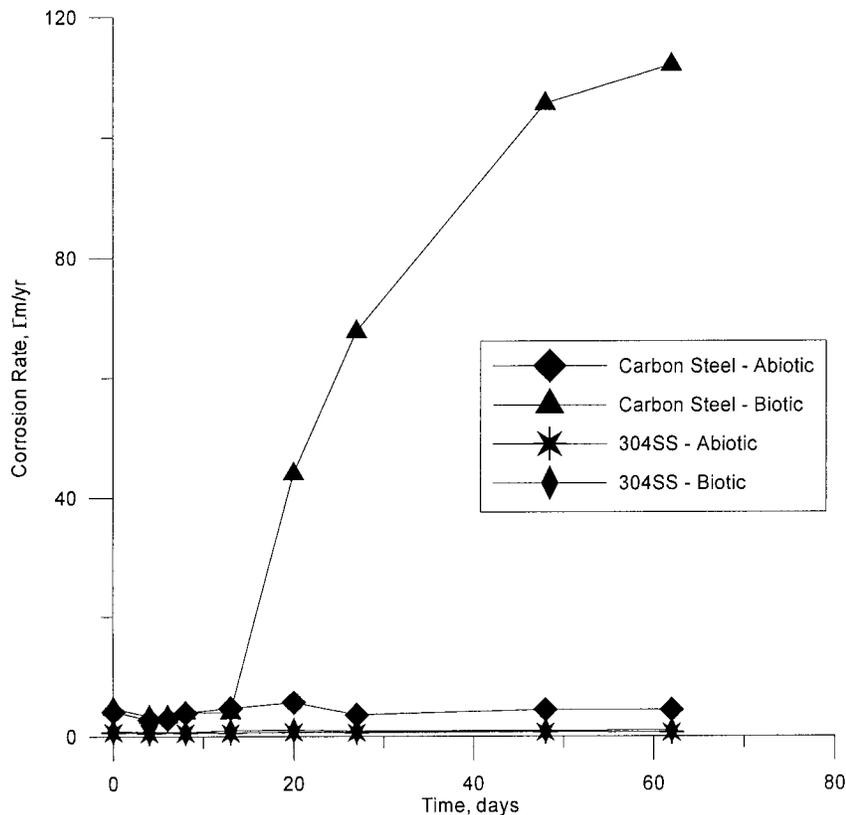
**Figure 8: Corrosion rates determined using linear polarization resistance.**
